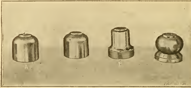
Fig. 24. An Example of "Air Spinning" and the Chucks used
