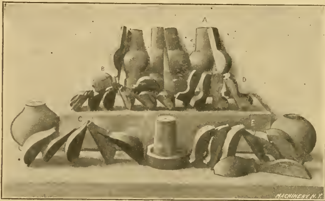
Fig. 29. Sectional Chucks made from Wood
