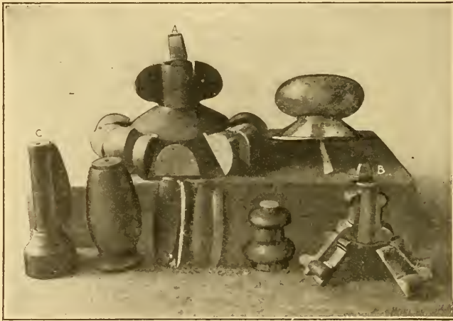
Fig. 30. Other Examples of Wooden Sectional Chucks
