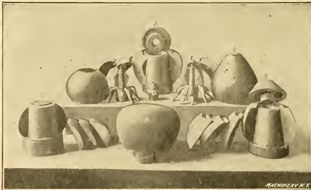
Fig. 28. A Group of Bronze Sectional Chucks
