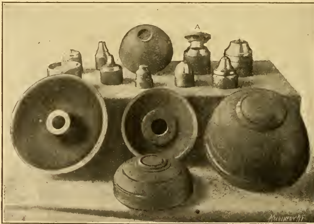
Fig. 25. Miscellaneous Collection of Spinning Chucks
